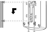
8. Press and lift out the handset holder, rotate it 180°, then snap it back into place so it holds the handset.
