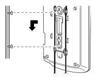
8. Press and lift out the handset holder, rotate it 180°, then snap it back into place so it holds the handset.
