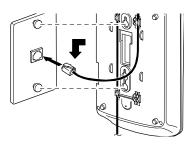
6. Press and lift out the handset holder, rotate it 180°, then snap it back into place so it holds the handset.
