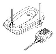
If the battery pack becomes completely discharged or the base loses power while the handset is away, the security access-protection code needs to be reset. To reset the code, return the handset to the base for about 5 seconds. If it was the handset that lost power, leave the handset on the base to recharge the battery pack
