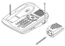
If the display is blank and the phone does not work, recharge the battery pack. (The battery power might be too low to light the display.)
