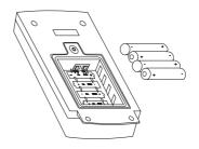
Use a flat blade screwdriver to loosen the screw in the transmitter's battery compartment cover, then lift the cover off.
