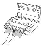
5. Replace the roller. Make sure the roller's tabs lock into place.
