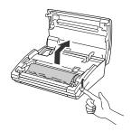
3. Press the roller's tabs outward and lift the roller out of the fax machine.
