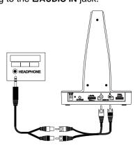
**Note:** To connect a Y-adapter to a <sup>1</sup>/<sub>4</sub>-inch headphone jack, slip the supplied <sup>1</sup>/<sub>4</sub>-inch adapter plug over the <sup>1</sup>/<sub>8</sub>-inch plug and complete the connections.
