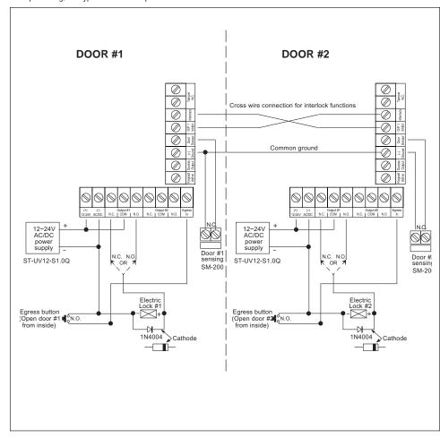
Interlock — Each keypad can be used as a stand-alone keypad. The mantrap feature is for a protected area with two doors to ensure only one door is open at a time. With the mantrap feature, when a user keys in the code to open one door, a signal is sent to the second keypad to disable it, thereby preventing access through the second door until the first door is closed.
