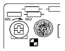
be increased by turning the control clockwise. Continue snapping the ruler on the window until the Yellow LED comes ON but the Red LED does not. Repeat this process with each window to ensure the **ENFORCER 190/190S** is set for every pane of glass.
