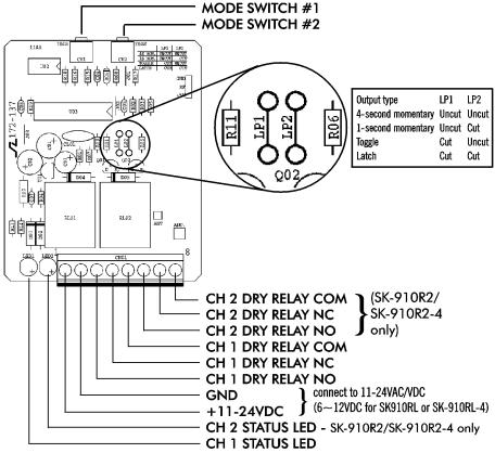
Mode Switch Operation (one per channel)
