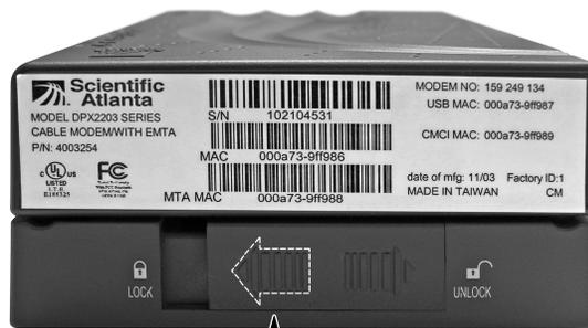
**3. Slide switch to left to lock into battery backup unit.**
