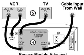
Bypass Module Attached to EXPLORER® 2000
