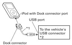
When connecting the iPod, remove a headphone cable from the iPod. When connecting the iPod, it is recommended to use a separately purchased car kit.
