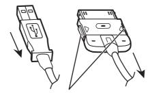
When disconnecting the iPod connector, grasp the connector firmly and pull it towards you.
