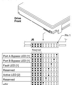
[1] The drive has a 2.2K ohm resistor in series with this LED driver. Connect the minus side of an external high-efficiency LED (i.e., 2ma) to this pin. Connect the plus side of the LED to +5V.
