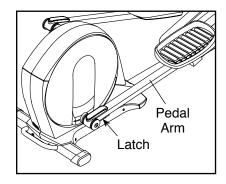
Next, raise the pedal arms until the magnets on the pedal arms touch the handlebars; the magnets will hold the pedal arms in place. Then, hold the handle and lift the frame until it locks in a vertical position.
