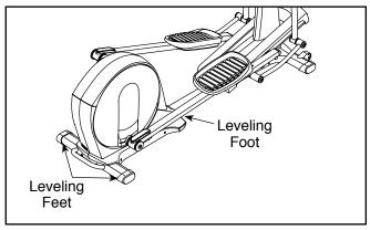
If the frame of the elliptical flexes during use, turn the center leveling foot until the flexing motion is eliminated.
