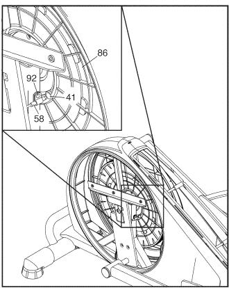
Next, rotate the Pulley (86) until a Magnet (41) is aligned with the Reed Switch (58). Slide the Reed Switch slightly toward or away from the Magnet. Then, retighten the M4 x 16mm Screw (92).
