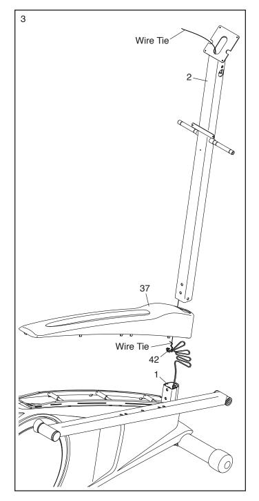
4. **Tip: Avoid pinching the Main Wire (42).** Slide the Upright (2) onto the Frame (1).
