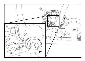
Next, turn the resistance knob to the lowest setting. With the left side shield removed, locate the Reed Switch (39). Turn the Crank (21) until the Magnet (38) is aligned with the Reed Switch. Loosen, but do not remove, the M4 x 15mm Screw (47). Slide the Reed
