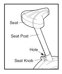
slide the seat post upward or downward and align one of the adjustment holes in the seat post with the indicated hole in the Frame. Insert the seat knob into the frame and the seat post, and turn the seat knob clockwise until it is tight. Make sure that the seat knob is inserted through one of the adjustment holes in the seat post.
