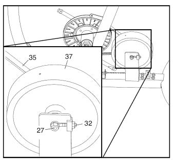
Next, loosen the two 3/8" Nuts (27), one on each side of the Flywheel (37). Then, tighten the M6 Nylon Locknuts (32), one on each side of the Flywheel, until the Belt (35) is properly tightened. Finally, tighten the Adjustment Nuts and reattach the side shields, the upright covers, and the pedals.
