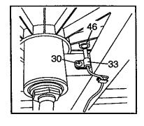
er to or away from the Magnet. Retighten the Screw. Turn the crank for a moment. Repeat until the console displays correct feedback. When the Reed Switch is correctly adjusted, reattach the left side shield.
