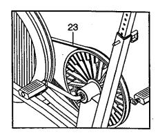
If the drive belt is properly adjusted, reattach the side shields. If the Belt needs to be adjusted, loosen the Axle Nut (29) on each side of the flywheel. To tighten the Belt, turn the Adjustment Nuts
