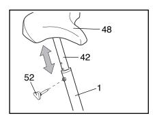
the Seat (48), dismount the exercise cycle, hold the Seat, and remove the Seat Knob (52). Raise or lower the Seat and insert the Seat Knob through the Frame (1) and the Seat Post (42). Tighten the Seat Knob into the welded nut on the Frame. **CAUTION:** Make sure to insert the Seat Pin through the Seat Post; do not insert the Seat Knob under the Seat Post.
