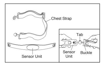
Next, wrap the heart rate monitor around your chest and attach the other end of the chest strap to the sensor unit. Adjust the length of the chest strap, if necessary.
