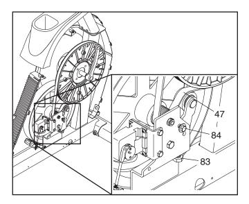
When the Drive Belt (47) is correctly adjusted, reattach the right shield, the right pedal, and the top shield and then plug in the power adapter.
