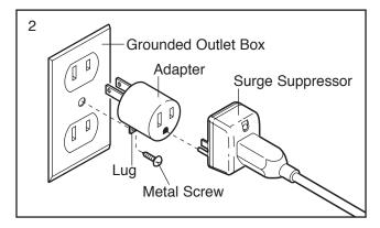
This product is for use on a nominal 120-volt circuit, and has a grounding plug that looks like the plug illustrated in drawing 1. A temporary adapter that looks like the adapter illustrated in drawing 2 may be used to connect the surge suppressor to a 2-pole receptacle as shown in drawing 2 if a properly grounded outlet is not available.
