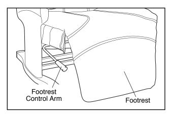
To lower the footrest, simply push the control arm forward.
