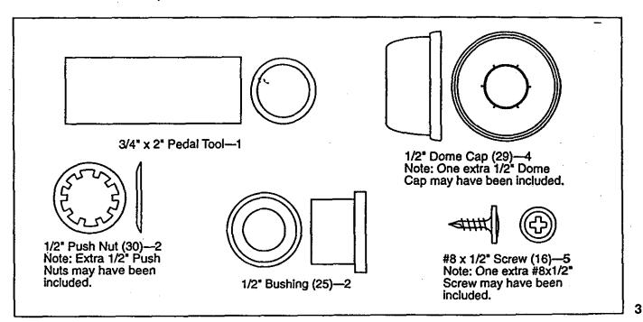
1. Tap a 1/2" Bushing (25) into each side of the Frame (6) as shown.
