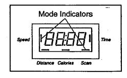
Speed, time, distance or calories mode—These modes can be selected by repeatedly pressing the mode button. The mode indicators will show which mode has been selected. The modes will be selected in the following order: speed, time, distance, calories.
