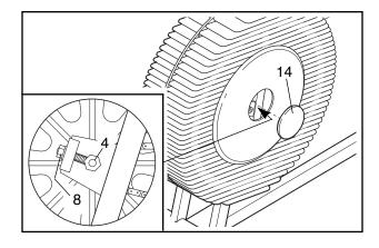
Pry the Access Cover (14) off the left side shield. Loosen the M8 Washer Nuts (4). To tighten the chain, turn the M6 Adjustment Nuts (8) clockwise; to loosen the chain, turn the Adjust-ment Nuts counterclockwise. Make sure that the fan is straight, tighten the Fan Nuts and reattach the Access Covers.
