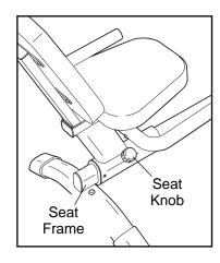
adjustment holes in the right side of the seat frame. Tighten the seat knob into the welded nut.
