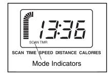
is selected, and a second mode indicator will show which mode is currently displayed. Note: If a different mode is selected, you can select the scan mode by repeatedly pressing the mode button. Time, speed, distance, or calories mode—To select one of these modes for continuous display, press the mode but-
