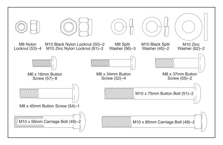
Identify the Front Stabilizer (2). Turn the Front Stabilizer so that the warning decal is in the position shown. While another person lifts the front of the Frame (1) slightly, attach the Front Stabilizer to the Frame with two M10 x 85mm Carriage Bolts (48) and two M10 Black Nylon Locknuts (50).
