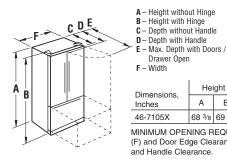
Clearance - Additional Width Required to Open the Doors 90° Left Hinge - Facing the refrigerator, handle is on your right and hinges are on your left. Right Hinge - Facing the refrigerator, handle
