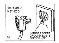
three-prong (grounding) wall outlet (Fig. 1) to minimize the possibility of electric shock hazard from this appliance.
