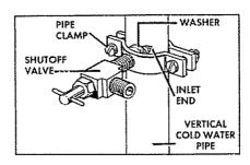
5. Fasten shutoff valve to cold water pipe with pipe clamp. Be sure inlet end is solidly in 3/16" drilled hole in water pipe and washer is under pipe clamp. Tighten packing nut. Tighten pipe clamp screws carefully and evenly so washer makes a watertight connection. Do not overtighten or you may crush copper tubing, especially if soft copper tubing is used. Now you are ready to connect the copper tubing.
