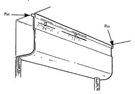
2. Pull the bottom of the light shield down and forward, then rotate the top up and off.
