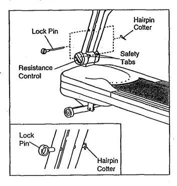
To use the upper body arms in the dual motion position, first make sure the resistance control is firmly tightened. Remove the lock pin from the upper body arms and the upright, and insert it through the safety tabs at the base of the upright. Insert the hairpin cotter into the lock pin.
