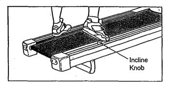
To increase the incline, stand with your left foot towards the back of the left foot rail as shown below. Using your right foot, press down the incline knob on the right foot rail, until the desired incline is reached. To decrease the incline, stand with your left foot towards the front of the left foot rail, and press down the incline knob until the desired incline is reached.
