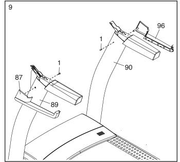
Tighten a #8 x 3/4" Screw (2) into the Left
