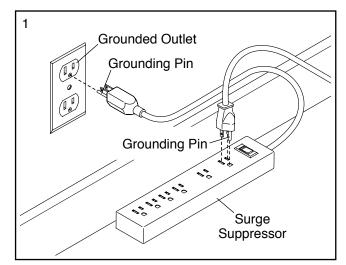
A temporary 2 adapter may be used to 00. connect the surge suppressor to a 2-pole receptacle if a properly arounded outlet is not available.
