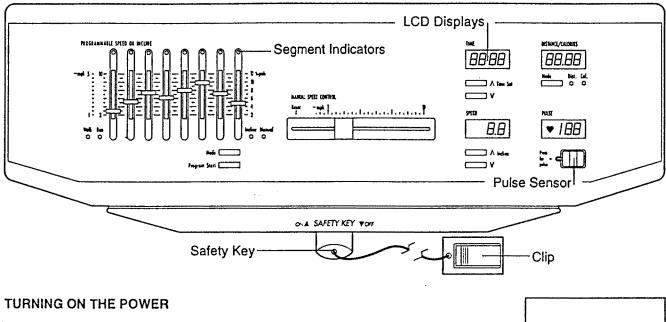
If the safety key is in the console, remove it. Make sure that the on/off switch located near the power cord is in the "on" position. Plug in the power cord (see PLUGGING IN THE POWER CORD on page 7.)
