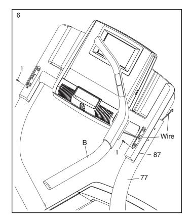
Set the right handrail assembly (B) onto the right Upright (77). Make sure that no wires are pinched. Attach the right handrail assembly with two 3/8" x 5 1/2" Screws (5) and two 3/8" Star Washers (8). Note: Start the lower Screw first.
