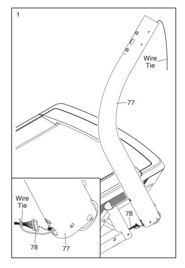
Attach the Upright (77) to the Base (80) with two 3/8" x 5 1/2" Screws (5), two 3/8" Star Washers (8), and a 3/8" x 2 3/4" Screw (17) with a 3/8" Star Washer (8) as shown. Start all three Screws, and then tighten them. Be careful not to pinch the Upright Wire (not shown) in the Upright.
