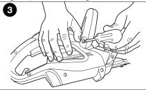
• For catalog number (79442, 51891) attach the handle and insert the threaded screw through the handle and housing as shown in **figure 4**.
