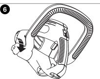
**NOTE:** The handle on the **79442, 51891** is adjustable to four different positions as shown **figure 7.** To move handle, unscrew plastic knob, position handle as desired and retighten knob.
