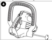
Insert the two screws into the holes shown in figure 5 and screw down. Do not over tighten.
