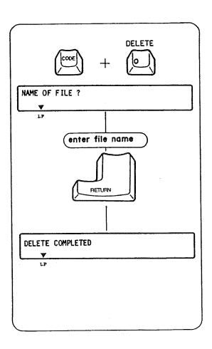
Use this function to delete any unnecessary files or to make room for new files in the memory.
