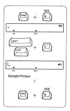
The symbols located at the upper right side of the three character keys can be typed with the following procedure.
