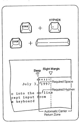
This function allows you to enter hyphens or spaces in the automatic carrier return zone that will not trigger the automatic carrier return.
