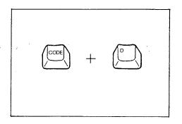
Hold down the Code Key and press the "D" Key. The typewriter will automatically perform a printout of features.
