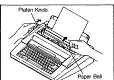
2) Turn the Platen Knob on the left of the typewriter to advance the paper. When the top of the paper comes into sight, pull the Paper Bail upward by hand to open it and continue turning the Platen Knob to feed paper in between the Paper Bail and Platen Roller.
