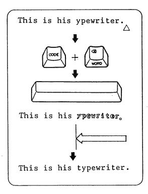
This function allows you to correct the last or previously typed word(s) only on the current line with one operation.
