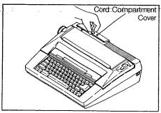
2) Press the mark on the Cord Compartment Cover on the rear of the typewriter, open the cover and take out the power cord.
