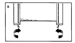
b. If the walking belt has shifted to the right, first remove the safety key and UNPLUG THE POWER CORD. Using the 3/16" allen wrench, turn the left rear roller adjustment bolt counterclockwise, and the right bolt clockwise, 1/4 of a turn each. Be careful not to overtighten the walking belt. Plug in the power cord, insert the safety key and run the treadmill for a few minutes. Repeat until the walking belt is centered.
