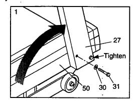
With the help of a second person, rotate the Left and Right Handrails (1, 11) up as shown. Insert two 3/8" x 1 1/4" Bolts (13) into the Left and Right Uprights (19, 27) and tighten the Bolts with the 7/32" Allen Wrench (90).
