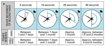
★ The second hand will resume normal movement after the indicated 5, 10, 20 or 30 seconds have elapsed.
