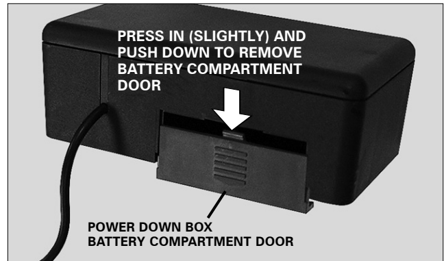
FIGURE 2: Receiver unit (power down box) battery compartment door removal.
