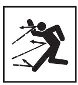
Soft tissue damage can occur from the compressed air stream.
