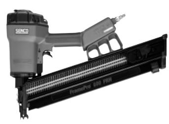
The FramePro® Full Round Head Nailers are the result of our award winning, feature loaded clipped head nailers now designed for Full Round Head nails. The FramePro® 600/650 FRH nailers feature an aggressive toenail safety, rugged aluminum casting, power to drive full round head nails from 2" to  $3\frac{1}{2}$ " in 5 gauges (.113 – .162) and an in-line magazine for superior balance and line of sight. All this and more for the Pro. Senco tools. Hard Work. Bring it On!
