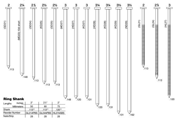
SECNO round head nails are designed to provide maximum fastening performance in partnership with the SN60, SN65, and SN65C. These quality nails are made to specs that meet codes and industry or manufacturer requirements. Check your SENCO rep or Authorized Dealer regarding availability of galvanized and Bright Basic
