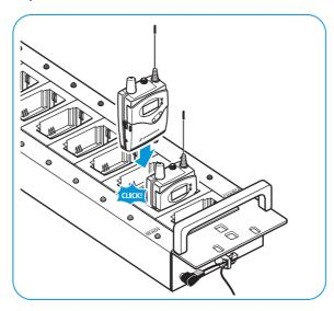
When an accupack is fully charged, the charging process stops automatically.
