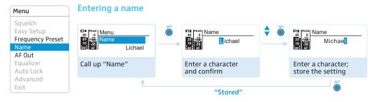
Via the "Name" menu item, you can enter a freely selectable name (e.g. the name of the performer) for the receiver.
