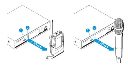
Press the synb button 1 on the receiver. "Sync" appears on the display panel of the receiver.
