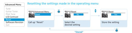
When resetting the settings made in the operating menu, only the selected settings for the pilot tone and for the frequency bank "U" remain unchanged. For an overview of the factory-preset default settings, refer to the supplied frequency information sheet.
