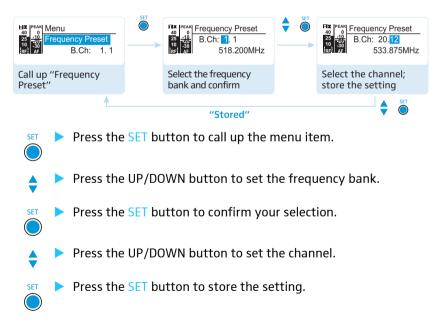
Squelch Easy Setup Frequency Preset Name AF Out Equalizer Auto Lock Advanced Exit
