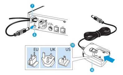
Only use the supplied NT 2-3 or NT 2-1 mains unit. It is designed for your receiver and ensures safe operation.
