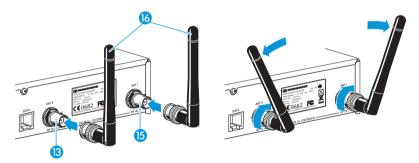
Align the rod antennas upwards in a V-shape.
