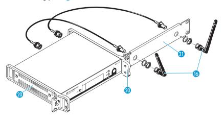
When using more than one receiver, we recommend connecting remote antennas and, if necessary, using Sennheiser antenna accessories. Fore more information, visit the ew G3 product page at www.sennheiser.com.
