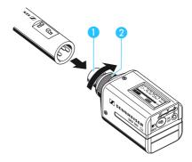
Tighten the locking ring 2 as shown.
