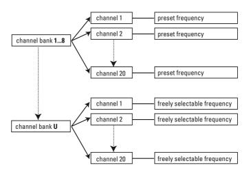
Each of the channels in the channel banks "1" to "8" has been factory-preset to a transmission frequency (see enclosed frequency table). These transmission frequencies cannot be changed but have been preset so that e.g. country-specific regulations on frequency usage are taken into account.
