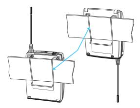
The clip is detachable so that you can also attach the transmitter with the antenna pointing downwards. To do so, withdraw the clip from its fixing points and attach it the other way round.
