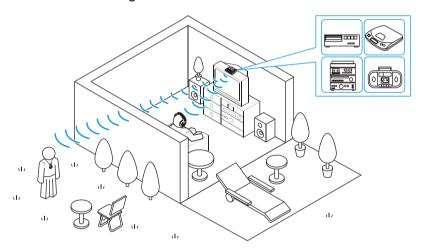
When the receiver leaves the range of the transmitter, it produces warning signals and then automatically switches off after 3 minutes.
