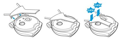
➤ Connect the induction loop ② to the socket ⑤ of the receiver.
