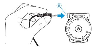
➤ Connect the 3.5 mm jack plug of the headphones to the socket ⑤ of the receiver.
