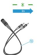
Plug the power supply unit ⑦ into a wall socket. The transmitter switches on. The multi-function LED ② flashes green after 9 seconds. The transmitter is in enrollment mode.
