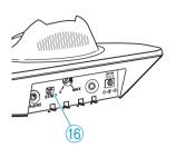
Set the ST/MO switch 16 on the transmitter to MO (mono).
