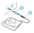
Plug the other end of the connection cable (19) into the head-phone socket on your sound source.
