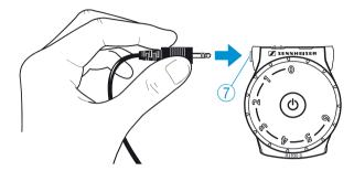
Connect the corresponding cable to the socket 7 on the receiver.
