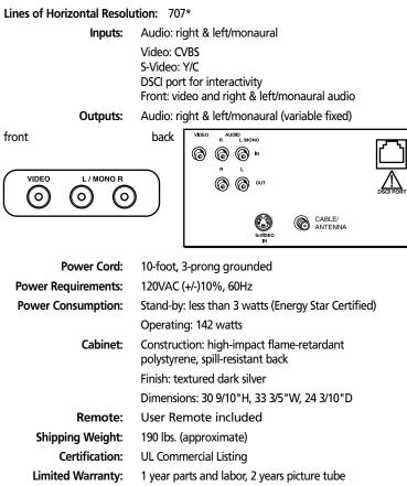
Lines per picture width based on EIA measurement criteria.
