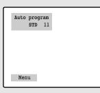
◄ The TV automatically cycles through all of the available channels and stores them in memory. This takes about one to two minutes. Press MENU•PROG at any time to interrupt the memorization process and return to the Channel menu.
