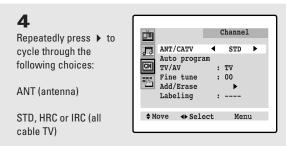
Note: STD, HRC and IRC identify various types of cable TV systems. Contact your local cable company to identify the type of cable system that exists in your particular area.
