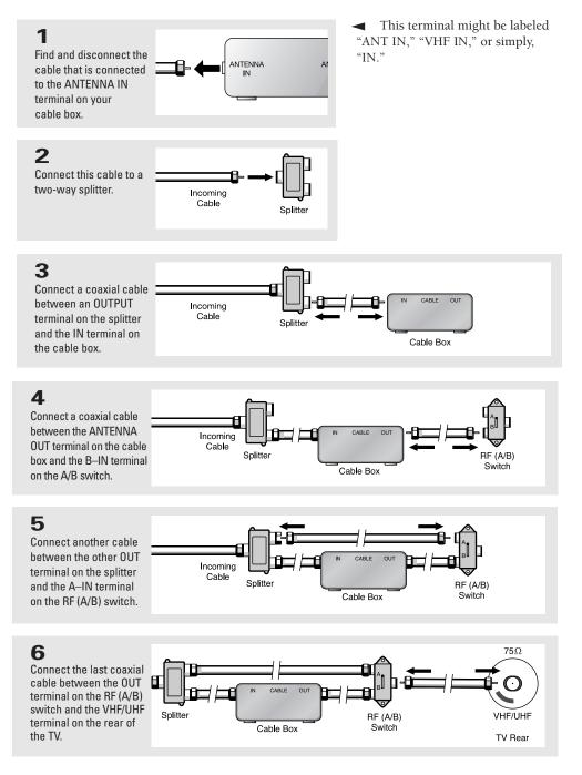
After you've made this connection, set the A/B switch to the "A" position for normal viewing. Set the A/B switch to the "B" position to view scrambled channels. (When you set the A/B switch to "B," you will need to tune your TV to the cable box's output channel, which is usually channel 3 or 4.)
