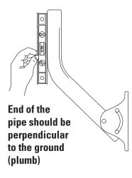
Secure the foot to its permanent location. Adjust the end of the pipe so that it is perpendicular to the ground. Tighten the hex nuts to hold the pipe in place.
