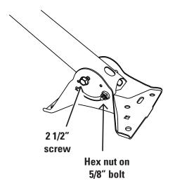
Find the end of the mounting pipe with holes on the sides for screws. Insert this end into the middle of the foot as illustrated here. Then insert the 2-1/2" screw through the foot and pipe as shown. Screw the 1/4" hex nut onto the end of the screw to hold the pipe and foot together. *Don't tighten the nut completely yet.*
