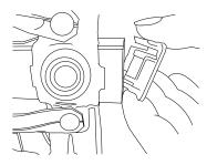
Insert the plastic end caps in the ends of the booms as shown here. Use a rubber mallet to gently tap them into the antenna booms to secure them.
