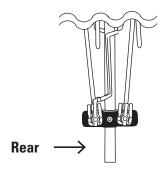
Starting from the rear of the antenna, unfold the elements on both the top and bottom of the antenna until they lock into place (as illustrated below). Make sure the elements are flat and parallel to each other when you've finished.
