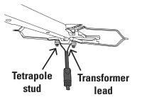
Use them to attach the transformer to the bottom of the antenna at the studs on tetrapole.
